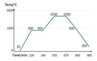
\*As always, the firing temperatures and times indicated are guidelines only and for different sintering furnaces, depending on their condition and calibration, these cycles will need to be adjusted accordingly. We recommend you run a trial firing to find the right temperature for your furnace.
